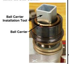
4. Using the 18" adjustable wrench, turn the Installation Tool counter clock-wise until the Ball Carrier is free from the body.
