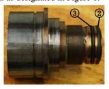
6. To re-assemble the Female Half, place the Spring on top of the Body.
