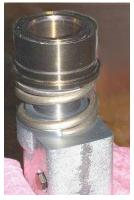
9. Using the Ball Carrier Installation Tool, tighten the Ball Carrier until there it meets the Body.
